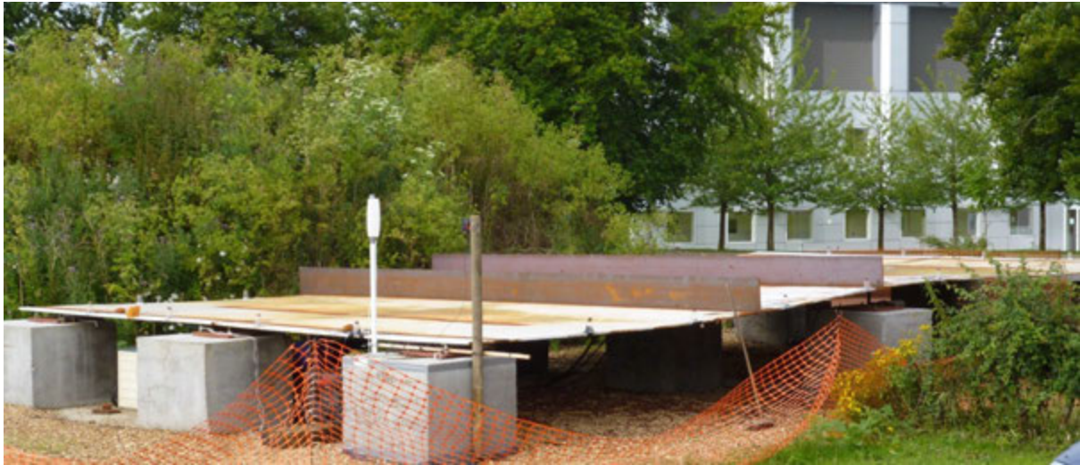
Figure 4. 12 x 6m plate specimen with stiffeners used for experiments for floor monitoring
